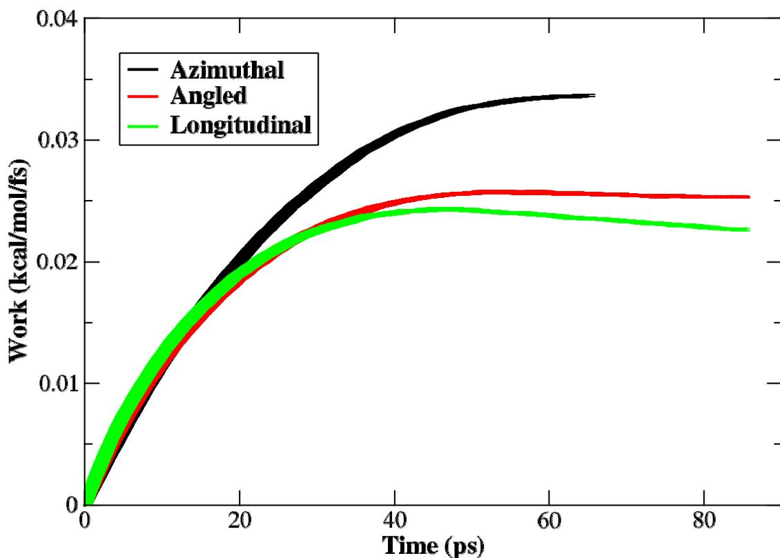
Figure S1: The calculated average work for the T<sub>m</sub> transitions per quasirepeat from the 25 ps 2 stage SMD. The work shown is the work of the virtual spring for each time step, with the width of the curve representative of the standard error. The azimuthal has the highest initial barrier, but is the shortest transition. The longitudinal has the lowest barrier, with the angled slightly higher than the longitudinal, but both take longer to reach the target endpoints than the azimuthal.
